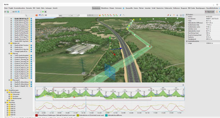
KorFin® Energy with real-time routing, including safety area and minimum distance control
