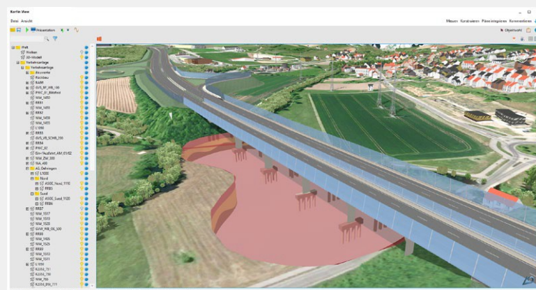
KorFin® overall model with substrate details for the foundation of bridge supports
