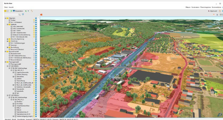
KorFin® overall model with the results of a sound immission calculation
