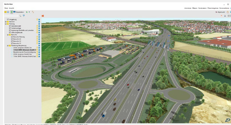
KorFin® overall model from as-built (hidden) and planning data with parameterized specialist objects
