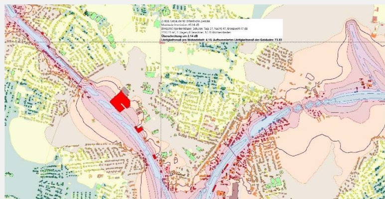
Building-specific noise evaluation in 2D
